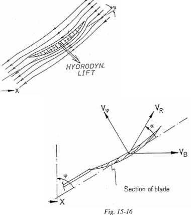
Because of the hydrodynamic shape of the blade profile presented to the water, thrust is produced at 90 degrees to the blade.
