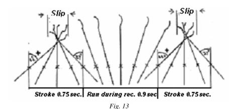
Figure 13 shows the real movement of the blade in relation to the boat. Considered in this way the former argument in respect of the efficiency of the arc angles, is less strong. The boat is moved past the blade rather than the blade past the boat.
