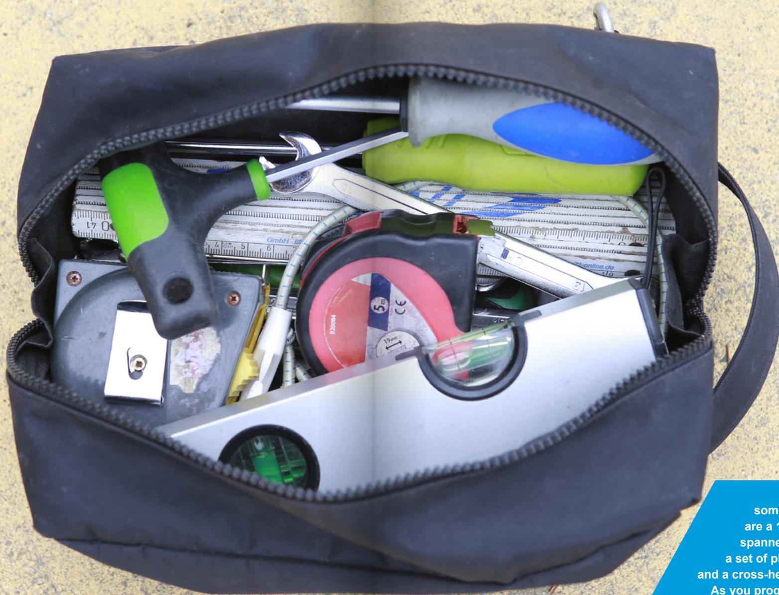
You will also need some tools: the basics are a 10mm and a 13mm spanner, a tape measure, a set of pliers, a flat-headed and a cross-headed screwdriver. As you progress you will want to add some specialist tools, a pitch gauge and a height stick.
