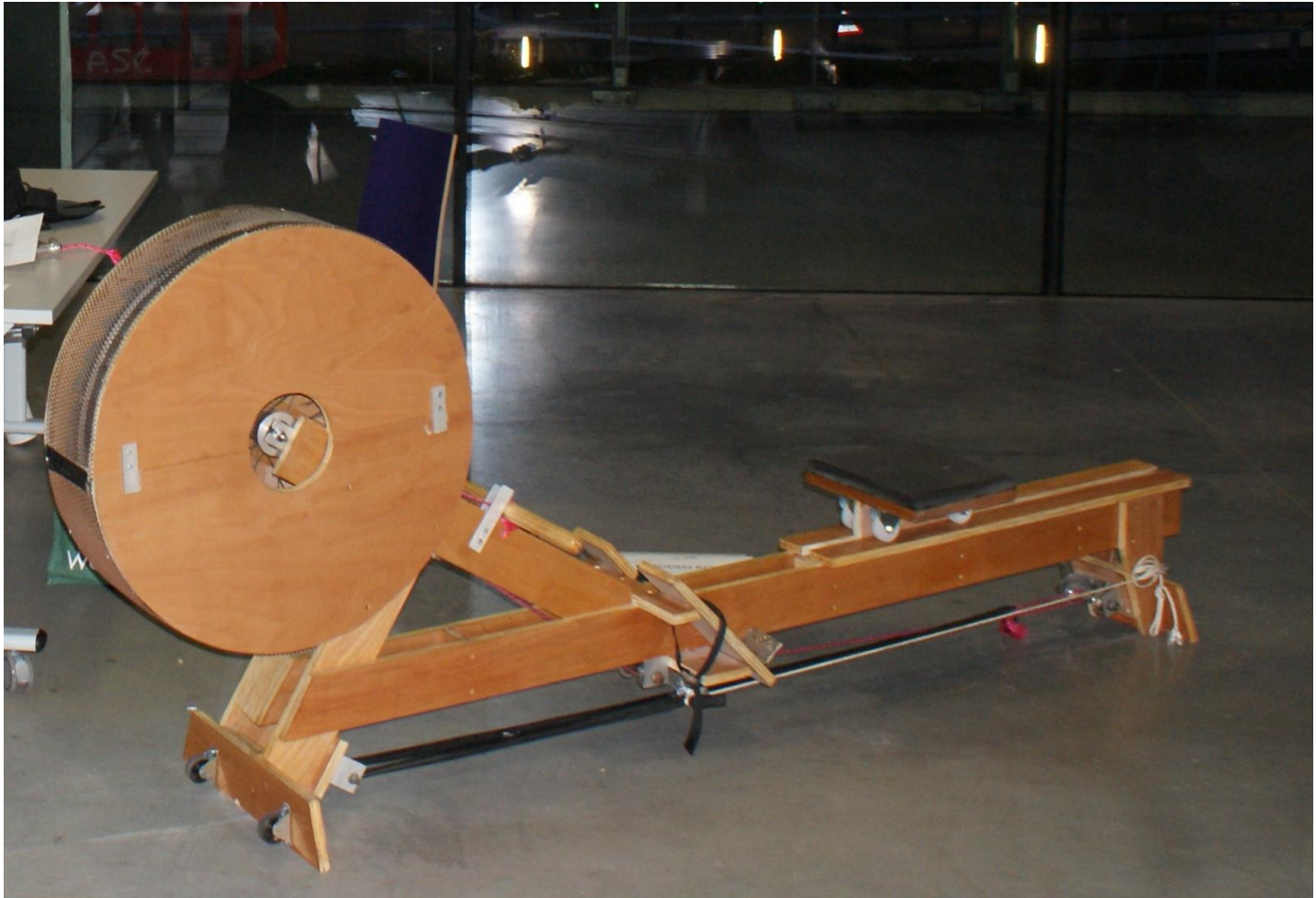
This one is for public use – so for safety, the impeller has a protective cover
