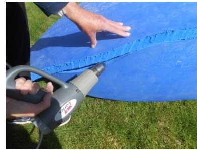
Welding the hull with a hot air gun
