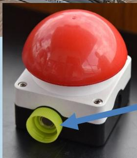
A new button was added to the “raising Start system” device which allows the lowering of all boots without actually giving start commands (prototype shown).
